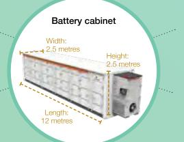
Likely to be lithium-ion battery packs enclosed in steel cabinets, similar to shipping containers
